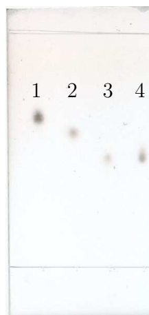
Figure 4.10: Separation of APGs with different alkyl chain lengths by TLC; RP-18 F_{254s} TLC plate, eluted by MeOH/water (9/1) and visualised by \text{H}_2\text{SO}_4 (200 g/L) . (1) \text{C}_8 - \beta -D-glucopyranoside; (2) \text{C}_{10} - \beta -D-glucopyranoside; (3) \text{C}_{12} - \beta -D-glucopyranoside; (4) \text{C}_{12} - \beta -D-maltoside.
