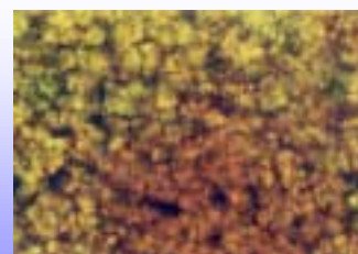
Polarizing microscopic image of the mesophase of TCQ-6C (Glassy, frozen LC phase)
